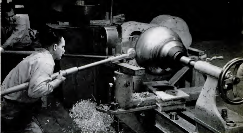
The tool end has a roller on it, and is controlled by the spinner. His helper (at upper left, above) controls long-handled fulcrum pin
